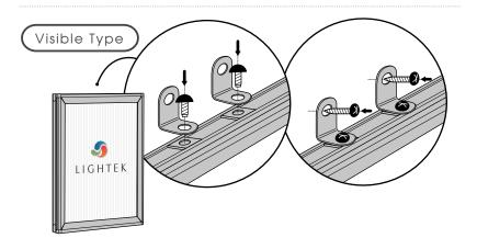
Step 1 Fix L bracket to the light box with screws.
