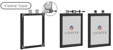
Step 1) Insert the supplied hanging clip into the groove on the top rear of the frame at approximately a 45° angle.
