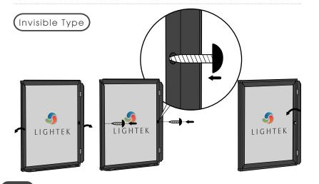
Step 1) Snap open frame sides to expose mounting holes in frame.
